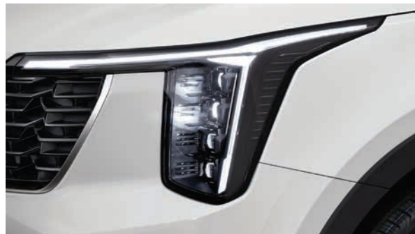
4-Cube Projection LED Headlamps with Sequential Turn Signals (SX Tech Pack Only)
