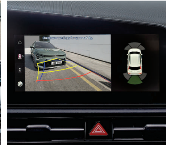
Rear View Monitor (RVM) The Rear View Monitor displays video of the situation behind the vehicle for safe parking.
