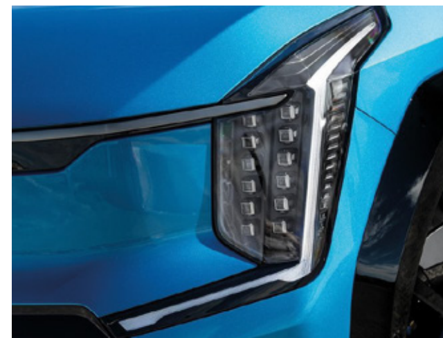
LED lighting (Small cube projection)
