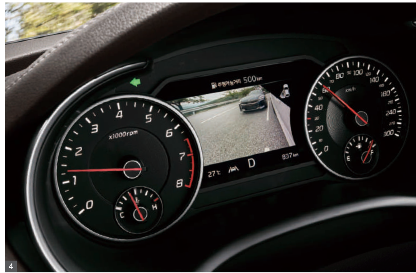
4 Blind-spot View Monitor (BVM) Cameras on the bottom of outside mirrors display a posterolateral view of the vehicle on the cluster's screen when the turn signal is activated, providing greater visibility of the surroundings in comparison to conventional outside mirrors for a safer driving environment.
