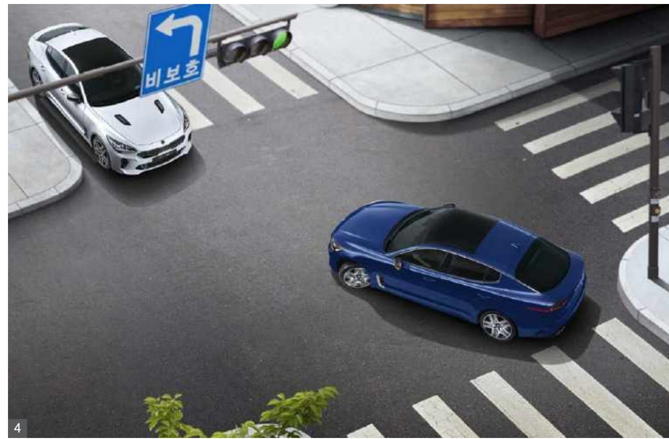
4 Forward Collision-avoidance Assist (FCA, oncoming traffic in intersections) Alerts the driver when danger of colliding with a car, pedestrian, or cyclist in front is detected. Automatically helps to apply the brakes if the risk of a collision increases even after sounding an alarm or when a risk of colliding with an oncoming vehicle on an opposite lane is detected while making a left turn in an intersection.
