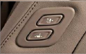
Front passenger walk-in device The driver can conveniently slide or incline the front passenger seat to facilitate access to the rear or front seats.
