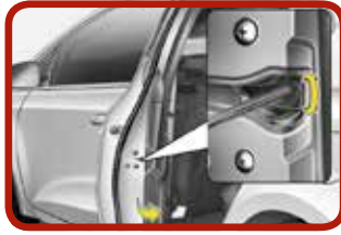
Locking doors in case of an emergency [4]
