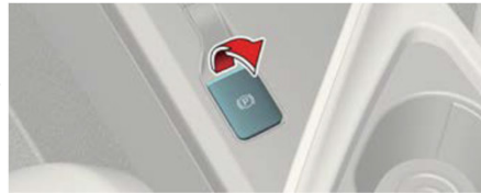
Set the Electronic Parking Brake (EPB)
