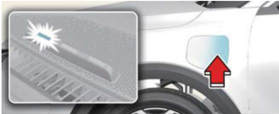
Operation of charging indicator lamp
