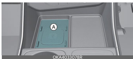
[A]: Charging pad
