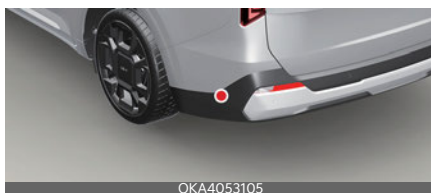
Rear side ultrasonic sensors
