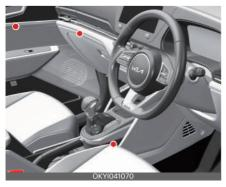
The ambient lights are applied to the front instrument panel, doors, and the centre console.
