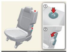
5. Back of the seatback will slightly go up, then lift up the 2nd row seat and set to upright position (vertical position).
