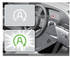
ISG system is indicated by AUTO STOP indicator (A) on the instrument cluster.
