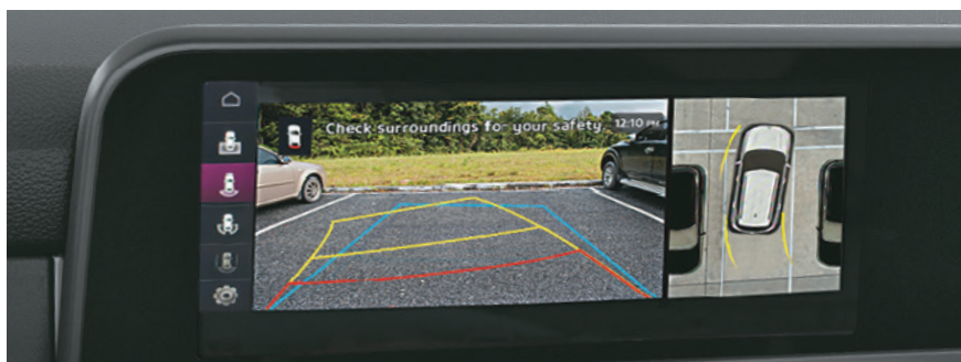
360° Camera with Blind View Monitor in Cluster
